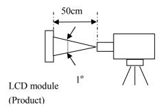
Luminance Meter (TOPCON BM-5A) Spectroradiometer (TOPCON SR-3)
