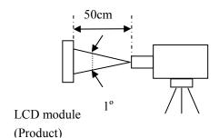
Luminance Meter (TOPCON BM-5A) Spectroradiometer(TOPCON SR-3)
