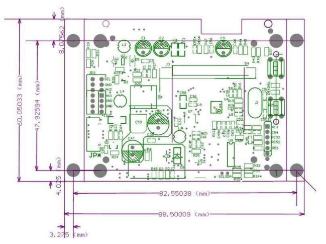
\*\*\*Note Some driver board Input video signal typePAL NTSC composite video 1Vvpp-75 Europe 4 Temperature -10 - +40 Degrees Input voltage 5.3V-18V, current is 130mA (12V).
