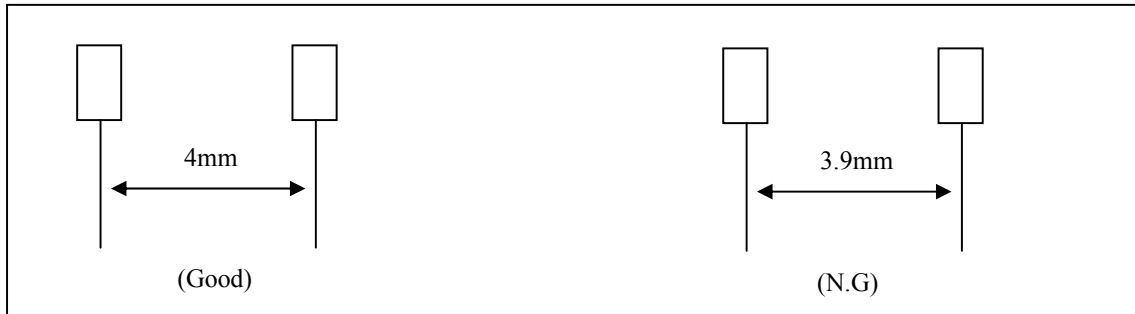
Fig 3. Minimum distance between dot defects [ Bright dot - to - Bright ]
