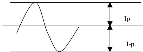
The degrees of unbalance =  $\frac{|I_p - I-p|}{I_{rms}} * 100(\%)$
