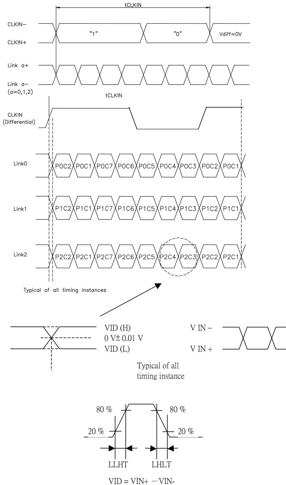
Parallel TTL Data Mapped to LVDS Receiver Inputs—DS90C384A
