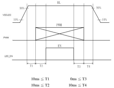
Note: The duty of LED dimming signal should be more than 20% in T2 and T3
