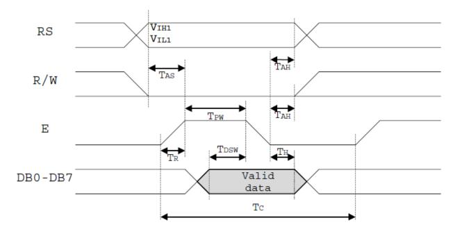
8.1.2 Reading data from ST7066 to MPU
