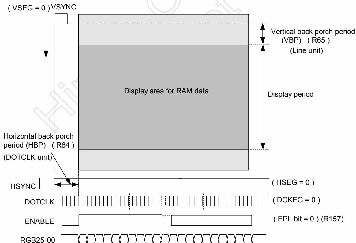
Figure 2. 8 RGB Interface Circuit Input Timing
