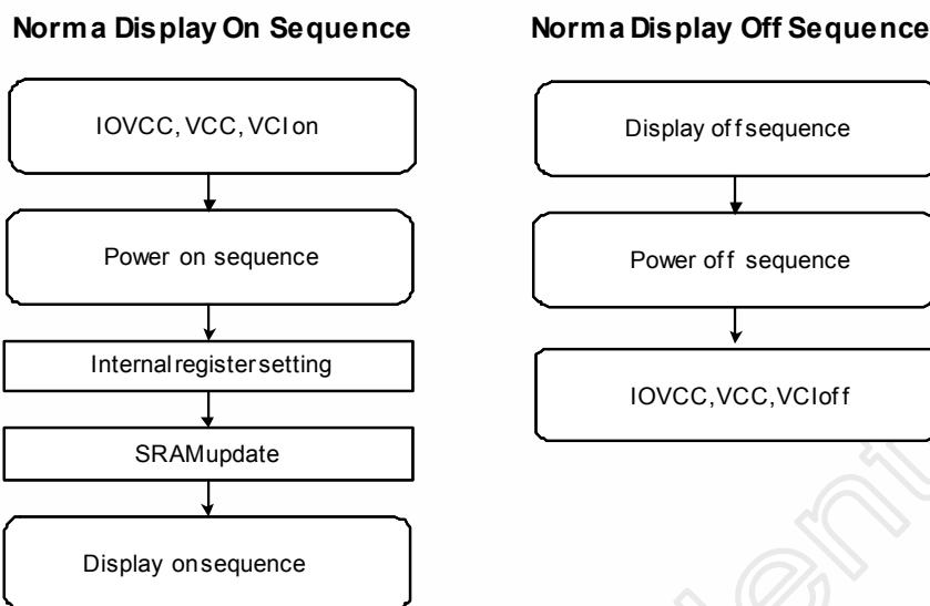
Figure 14. 1 Normal Display On / Off Sequence
