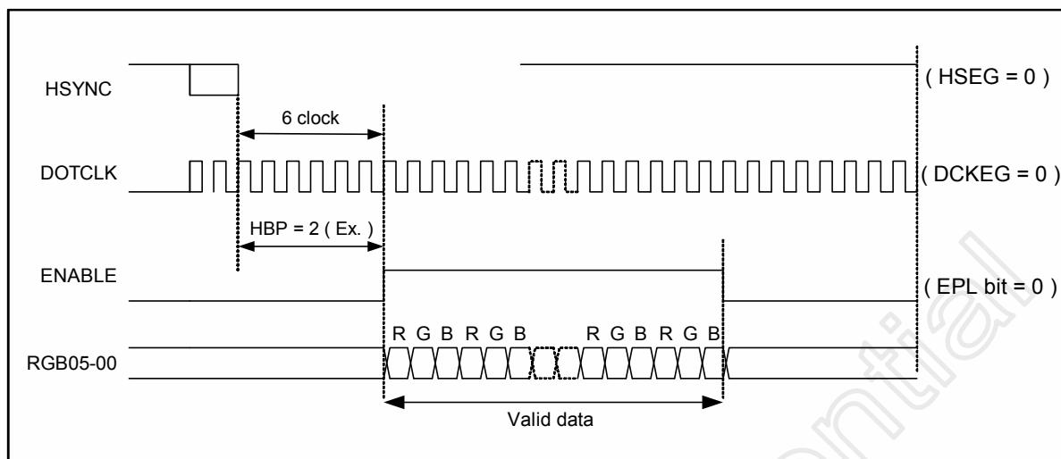
Figure 2.9 RGB3 Type (6-bit Interface Mode) Input Timing
