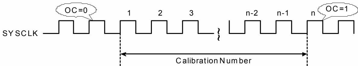
Figure 3. 9 Adjust by Calibration
