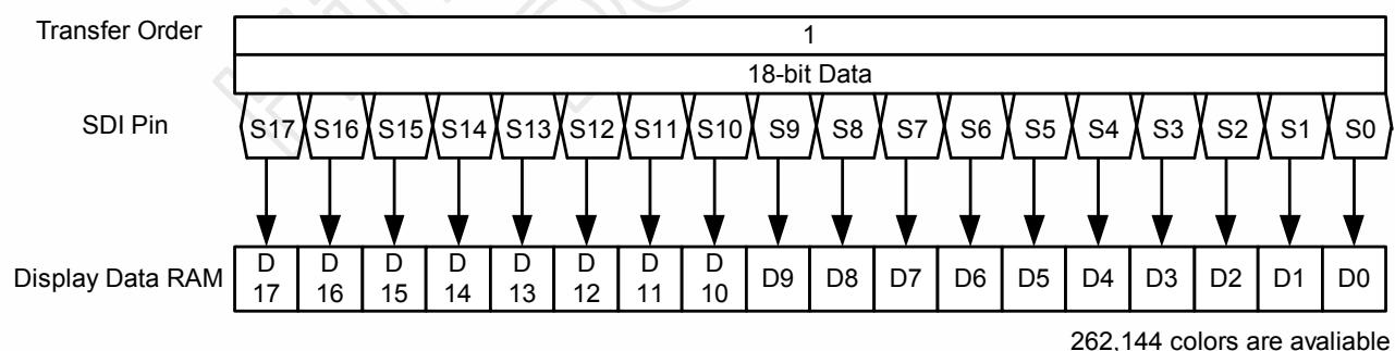
**(9) MPU9 Type (16-bit serial)**
