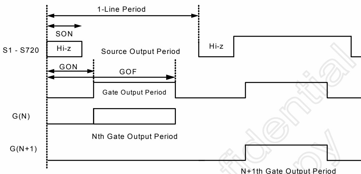
Figure 10. 1 Display Driving Period Time Setting
