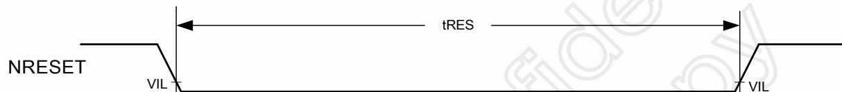
Figure 17. 6 Reset Timing
