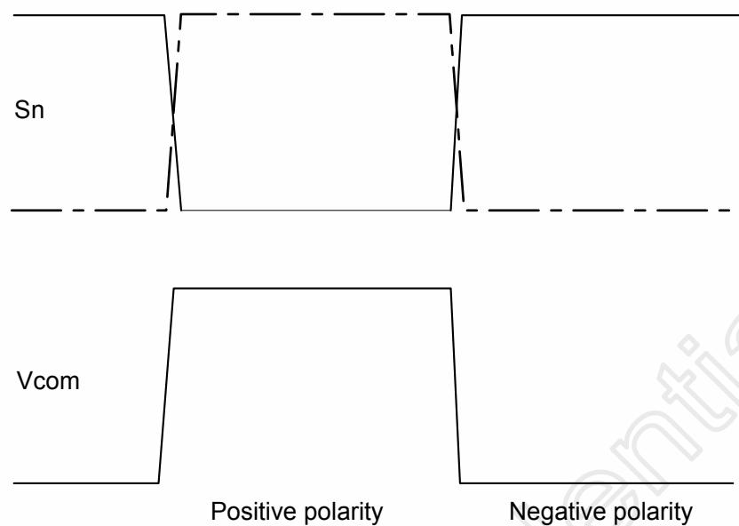
**Figure 8. 4 Relationship between Source Output and Vcom**
