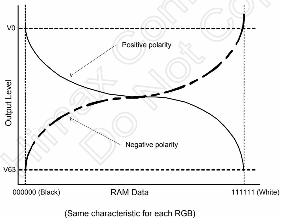
**Figure 8. 5 Relationship between GRAM Data and Output Level (REV = 1)**
