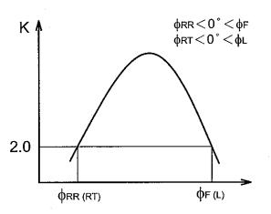
Contrast ratio K vs viewing angle  $\phi$
