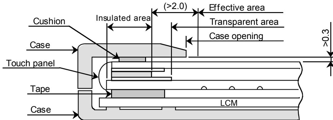
(2) The clearance between the touch panel and the case shall be designed so that the case edge never presses the input screen when it is deformed by heat or other causes.
