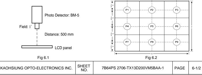
Note 3: The Contrast Ratio is measured from the center point of the panel, P5, and defined as the following equation:
