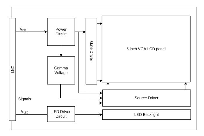
Note 1: Signals are DCLK, DE, and RGB data bus.
