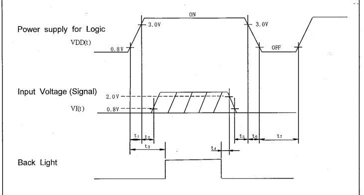
$\begin{array}{ccc} \underline{\text{POWER ON}} & & & \\ & & t_1 \leq & 15\,\text{ms} \\ & & 0\,\text{ms} < t_2 \leq & 45\,\text{ms} \\ & 0. \ 1s \leq & t_3 \end{array}$
