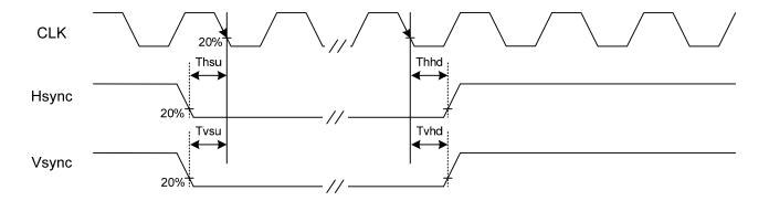
Fig. 9.6 Setup & Hold Time
