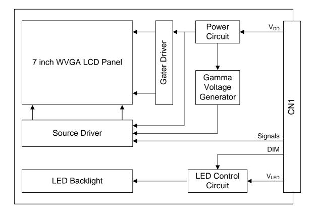
Note 1: Signals are a DE, Hsync, Vsync, CLK and RGB data bus.
