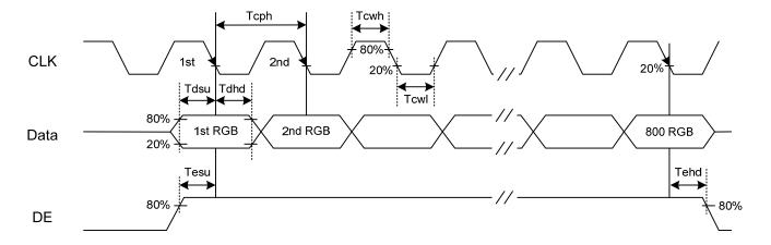
Fig. 9.5 Setup & Hold Time
