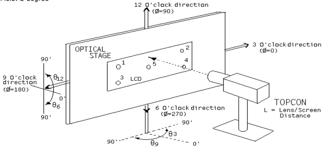
**Figure 2. Average Luminance Measurement Locations & Uniformity Measurement Locations**
