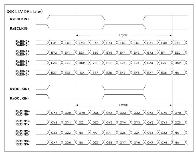
Note: X/Y/Z data 7: MSB, X/Y/Z data 0: LSB, DSP = DSPTMG, V-S = Vsync, H-S = Hsync
