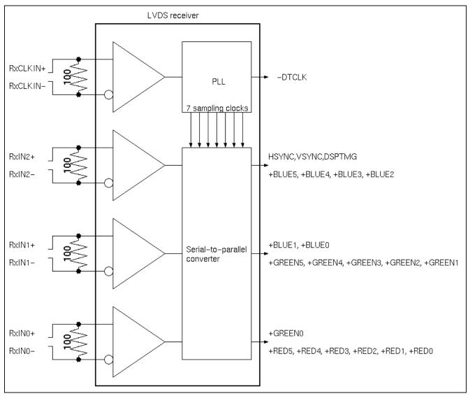
The module uses a 100ohm resistor between positive and negative lines of each LVDS signal input.
