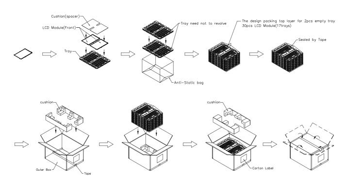
Figure. 7-1 Packing method
