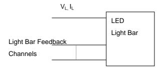
Note (2) For better LED light bar driving quality, it is recommended to utilize the adaptive boost converter with current balancing function to drive LED light-bar.
