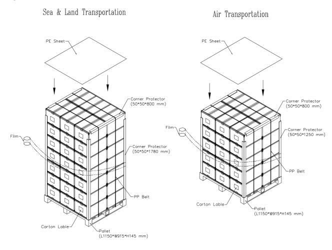
Figure. 7-2 Packing method
