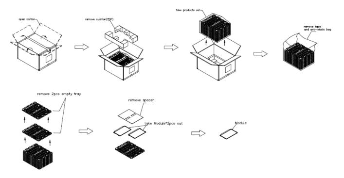
Figure. 7-3 Un-Packing method
