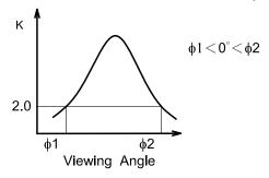
Contrast ratio K vs viewing angle  $\phi$
