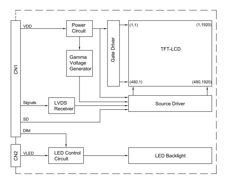
Note: Signals are CLK, and pixel data pairs.
