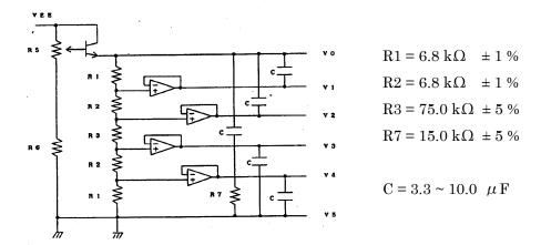
These value above are theoretically calculated. Fine tuning might be required in some cases. For fine tuning value of the resistor shall be adjust to conform with the following equation.
