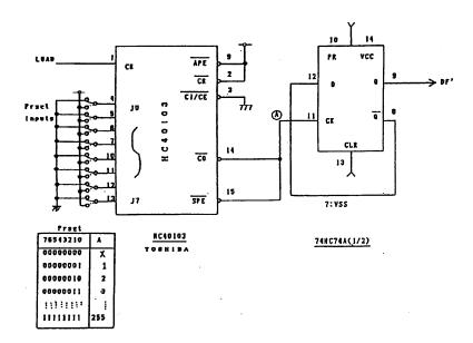
There may be flickering on screen according to some LOAD signal frequencies. If in happens, set PRSET INPUTS terminals to select optimized conditions.
