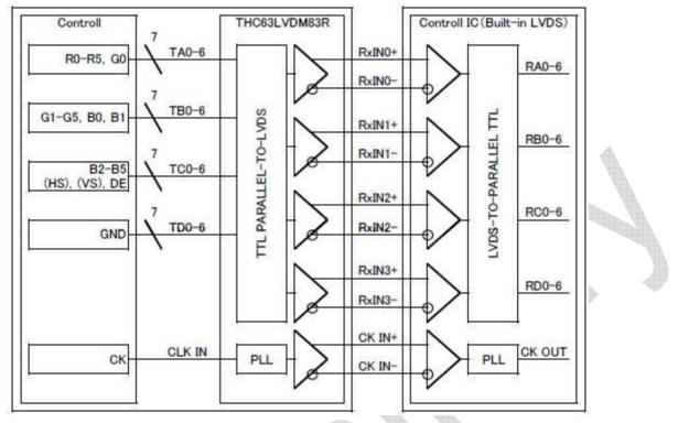
When using "6-bit Transmitter", please connect the unused channel of the control IC receiver as described in the diagram below.
