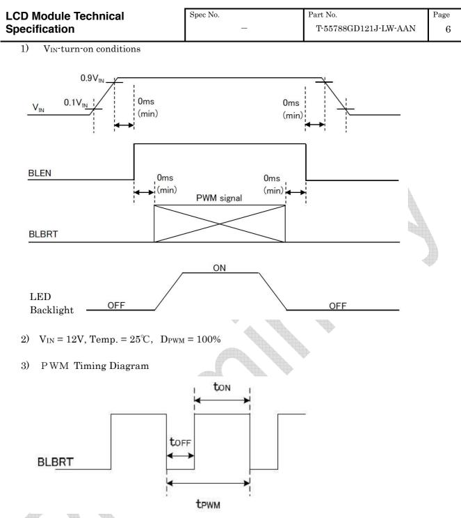
ton, toff  $\geq 50 \,\mu$  s. In case of lower frequency, the deterioration of the display quality, flicker etc., may occur.
