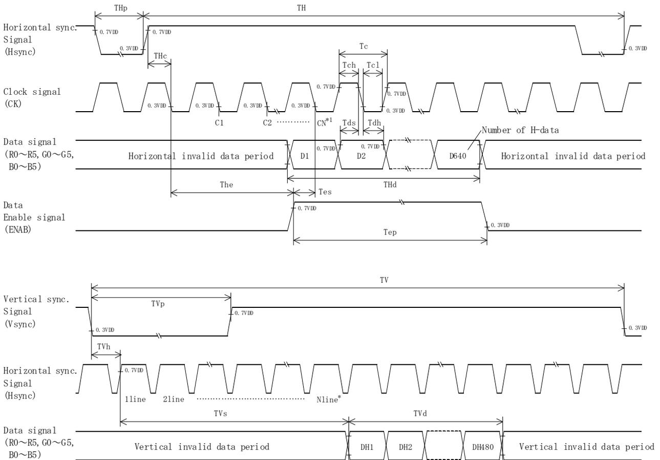
\*1 When ENAB is fixed "Low" the display starts from the data of C104(Clock).
