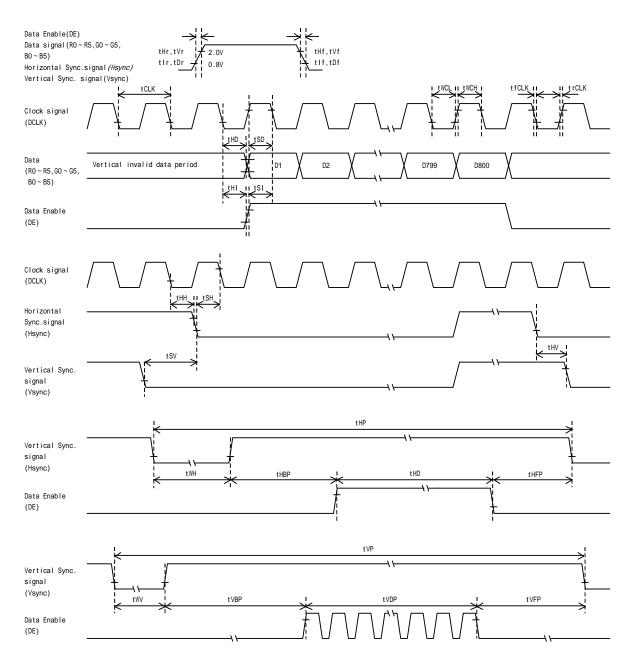
8-3. Input Data Signals and Display position on the screen
