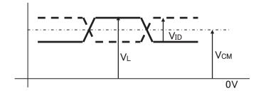
5)  $V_{CM}$ : LVDS Common mode voltage ( $V_{CM}$ =1.25V)
