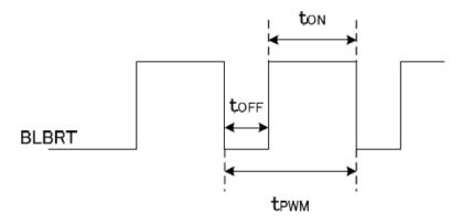
ton, toff  $\geq 50 \,\mu$  s. In case of lower frequency, the deterioration of the display quality, flicker etc., may occur.
