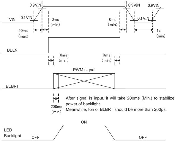
2)  $V_{IN} = 12V$ , Temp. = 25°C,  $D_{PWM} = 100\%$
