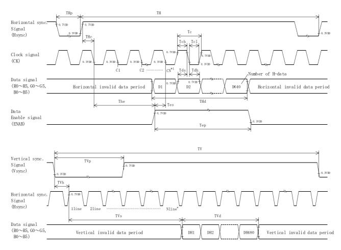
\*1 When ENAB is fixed "Low" the display starts from the data of C104(Clock).
