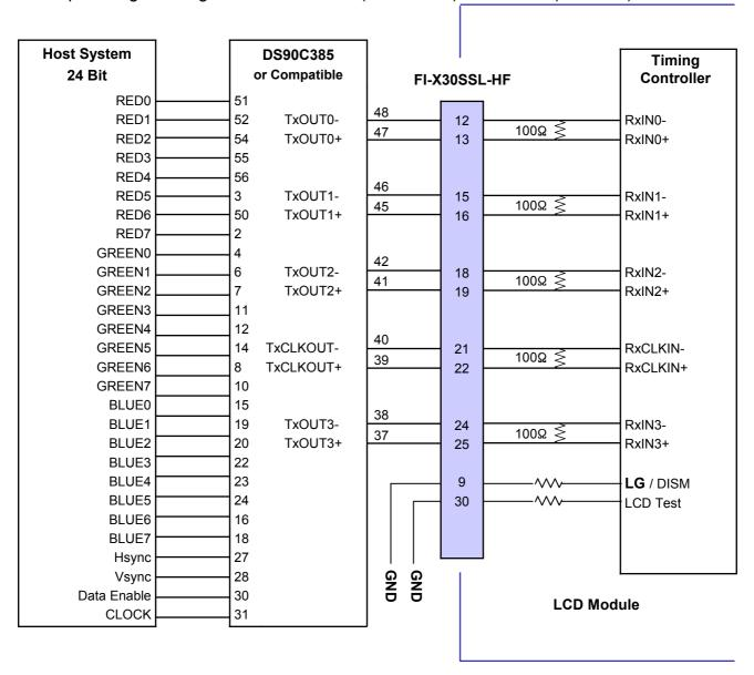
Note: 1. The LCD Module uses a 100  $Ohm[\Omega]$  resistor between positive and negative lines of each receiver input.
