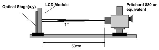
FIG. 1 Optical Characteristic Measurement Equipment and Method
