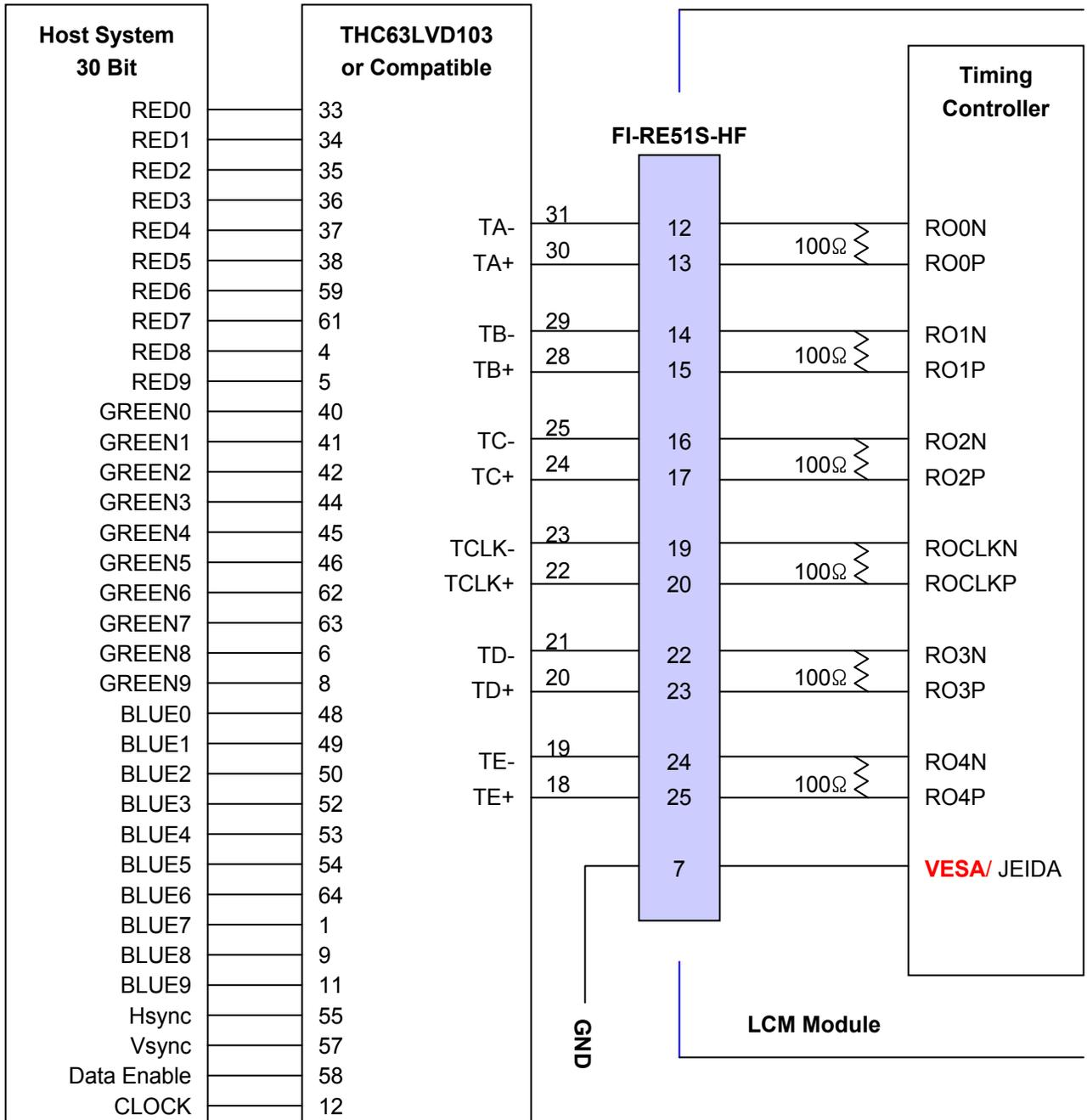
Note: 1. The LCD module uses a 100 Ohm[Ω] resistor between positive and negative lines of each receiver input.
