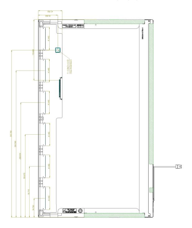
In order to avoid IC damage, it is not allowed to have such overlappings as cables or antennas, camera, WLAN, WWAN over these COF locations.
