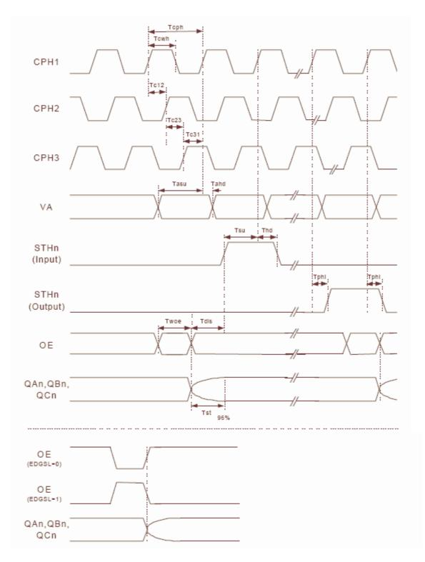
• Remark : The sample-and-hold circuits are switched and the outputs are started with new data at the rising or falling edge of OE.
