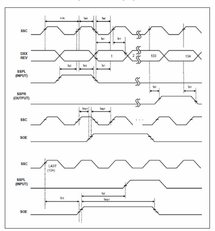
Fig. 2 Gate D-IC Timing Diagram
