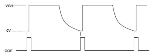
[Note 6-1.3] V<sub>IH</sub> = DVDD, V<sub>IL</sub> = GND, SOE Pulse Width = 2.87us, fclk = 8.005MHz, AVDD = 5V, Recommended Gamma Correction Voltage, with Probe Load.
