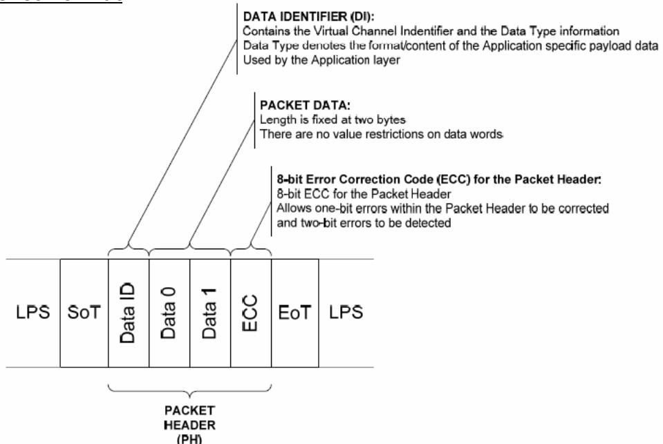
A Short packet shall contain an 8-bit Data ID followed by two command or data bytes and an 8-bit ECC; a Packet Footer shall not be present. Short packet shall be four bytes in length.
