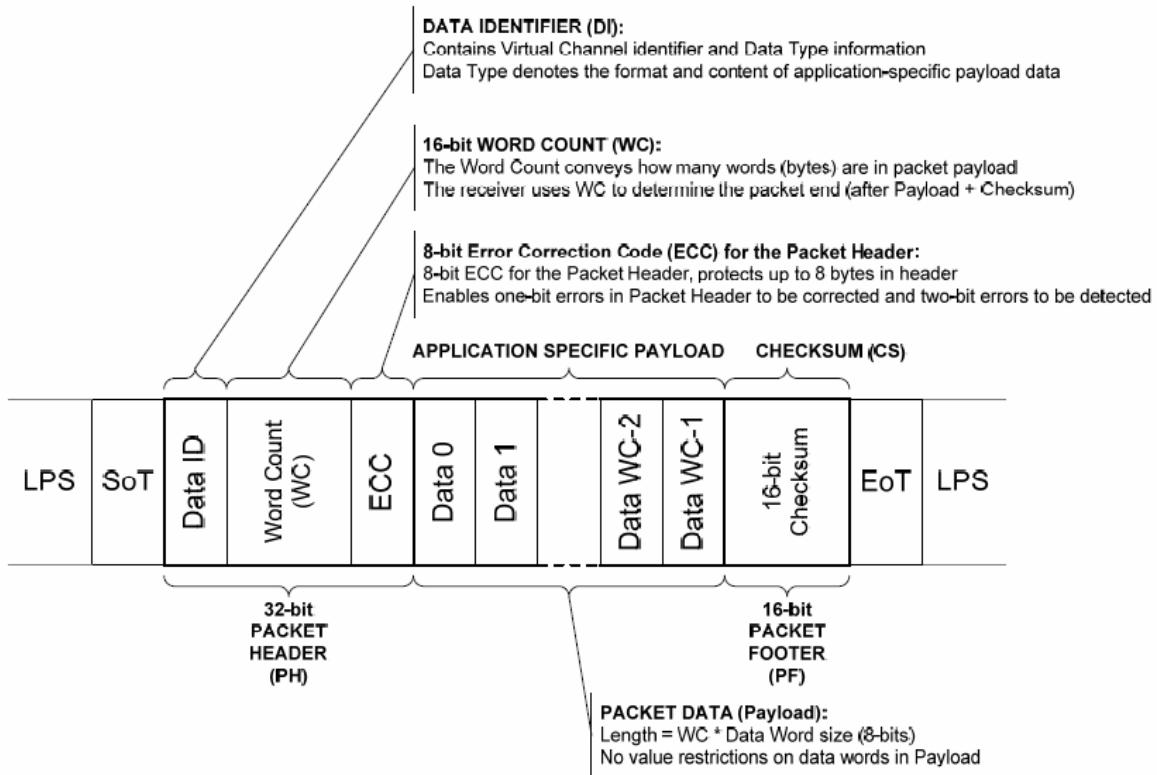
A long packet shall consist of three elements : a 32-bit Packet Header (PH), an application-specific Data Payload with a variable number of bytes, and a 16-bit Packet Footer (PF).
