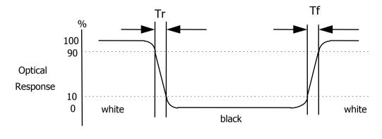
\* Voltage conditions for Response time Vgate : 19V DC Vdata : 0V~3.3V DC Vcom : 0V (Ground)
