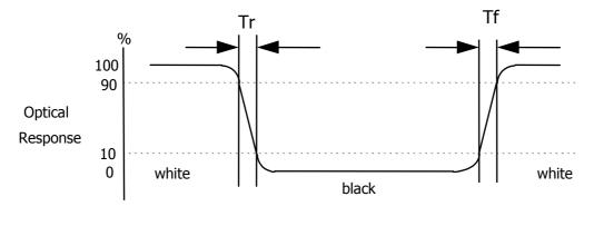
\* Voltage conditions for Response time Vgate : 19V DC Vdata : 0V~3.3V DC Vcom : 0V (Ground)
