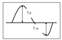
\* Asymmetry rate:  $|I_p - I_{-p}| / I_{rms} * 100\%$ \* Distortion rate  $I_p (or I_{-p}) / I_{rms}$
