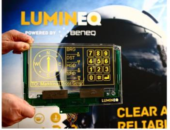
The ELT256.120.90 is a TASEL transparent matrix display designed for use in applications requiring full see-through properties of the display, be that for functional or aesthetic reasons.
