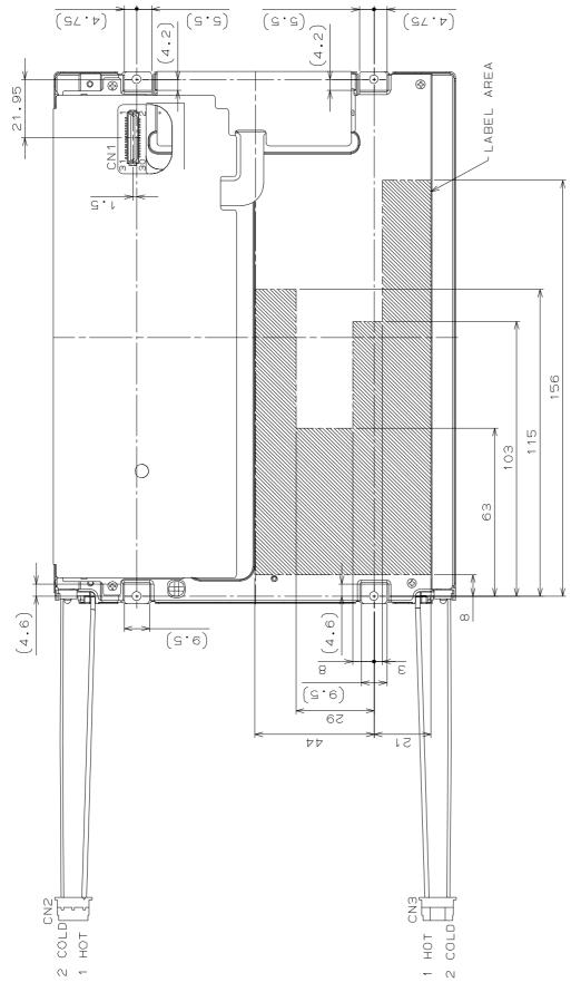
1)Tolerance is ±0.5mm unless noted. 2)Thickness of PET film is not included. 3)Third angle projection
