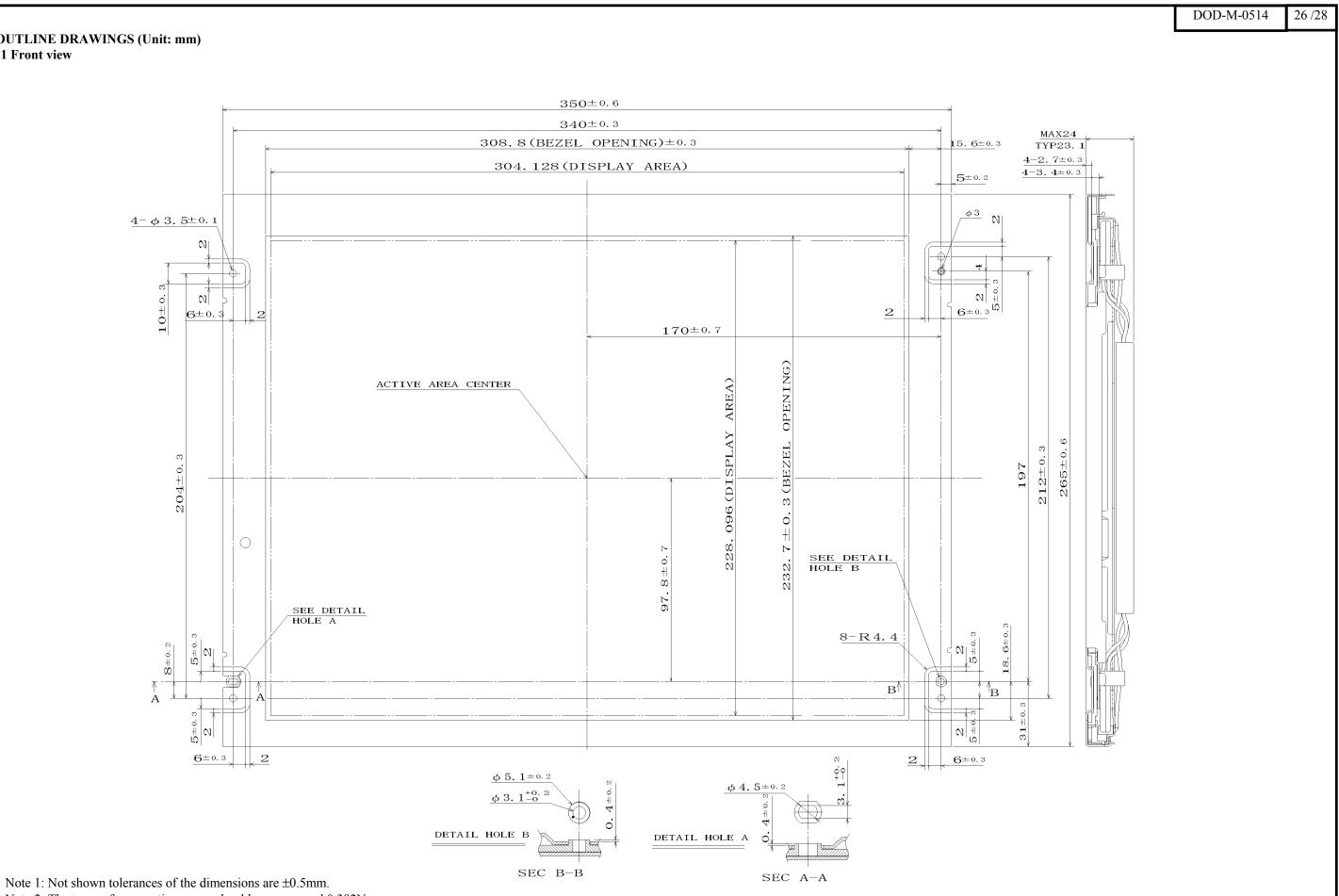
Note 2: The torque for mounting screw should never exceed 0.392N·m.
