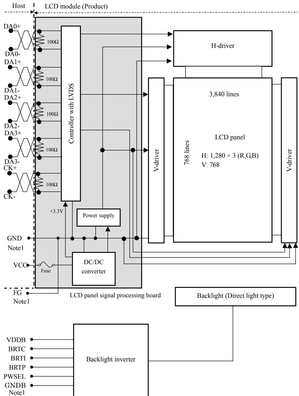
Note 1: GND is connected to FG (Frame ground). GNDB is not connected to FG.
