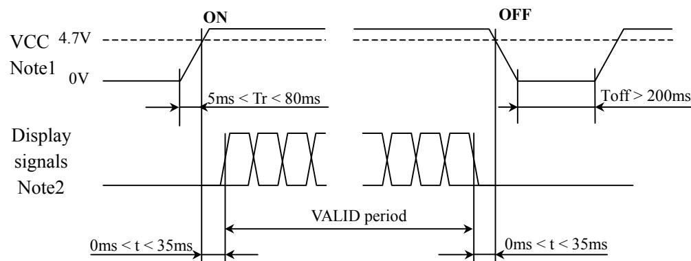
Note1: In terms of voltage variation (voltage drop) while VCC rising edge is below 4.7V, a protection circuit may work, and then this product may not work.
