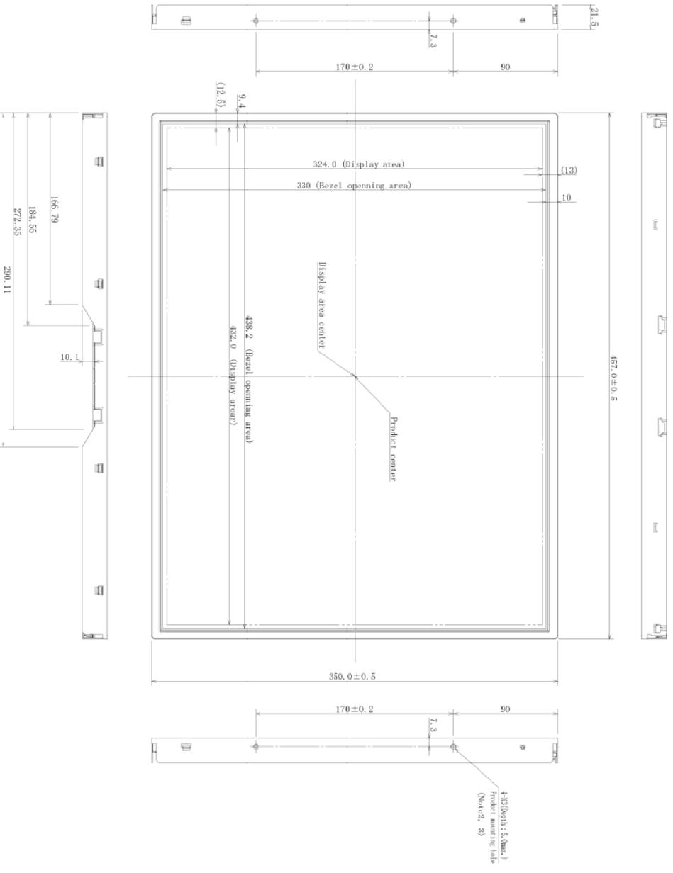
Note1: Not shown tolerances of the dimensions are  $\pm 0.5$ mm.
