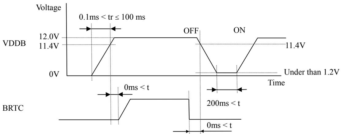
Note1: If  $tr$  is more than 100 ms, the backlight will be turned off by a protection circuit for LED driver board.
