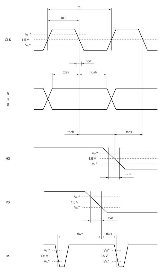
\* V  $_{\text{IH}} = 3.15$  V (min.) to 5.00 V (max.) V  $_{\text{IL}} = 0.00$  V (min.) to 0.90 V (max.)
