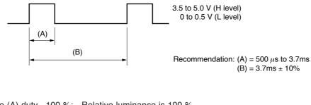
Pulse (A) duty100 %:Relative luminance is 100 %Pulse (A) duty20 %:Relative luminance is 10 % (reference value)
