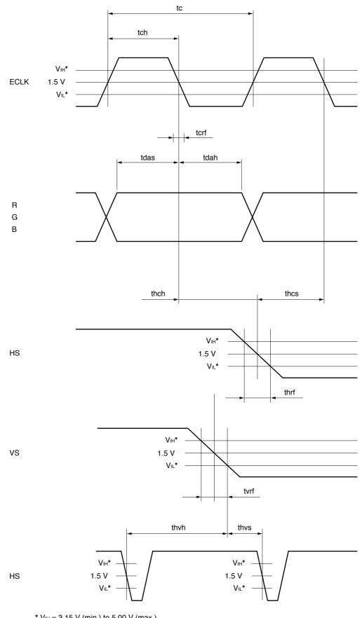
\* V\_{IH} = 3.15 V (min.) to 5.00 V (max.) V\_{IL} = 0.00 V (min.) to 0.90 V (max.)
