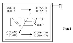
Figure 1. Normal scan (DPS: Low or Open)
