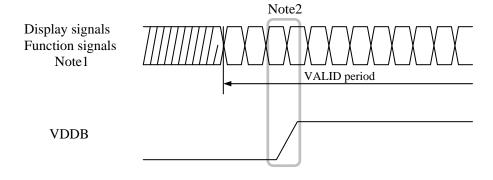
Note1: These are the display and function signals for LCD panel signal processing board.
