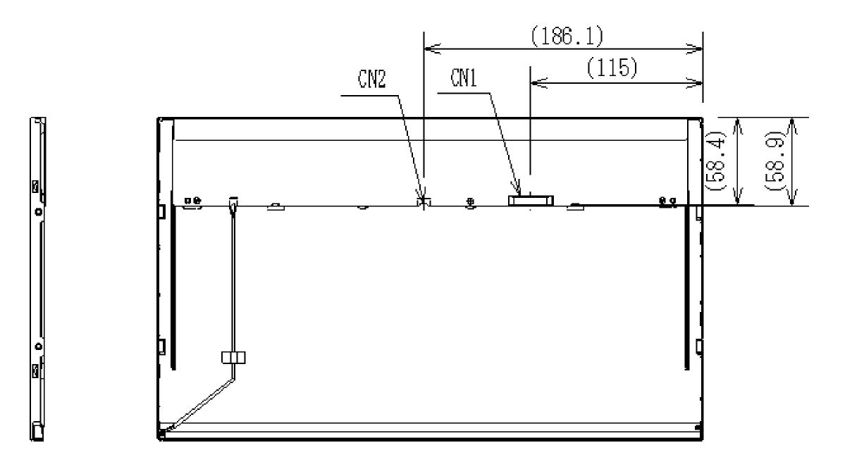
Note1: The values in parentheses are for reference. Note2: The torque for product mounting screws must never exceed 0.34N·m. 2
