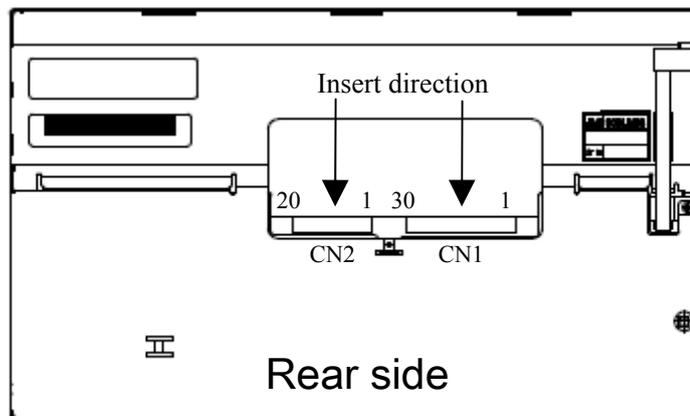
4.5.3 Connection between receiver and transmitter for LVDS
