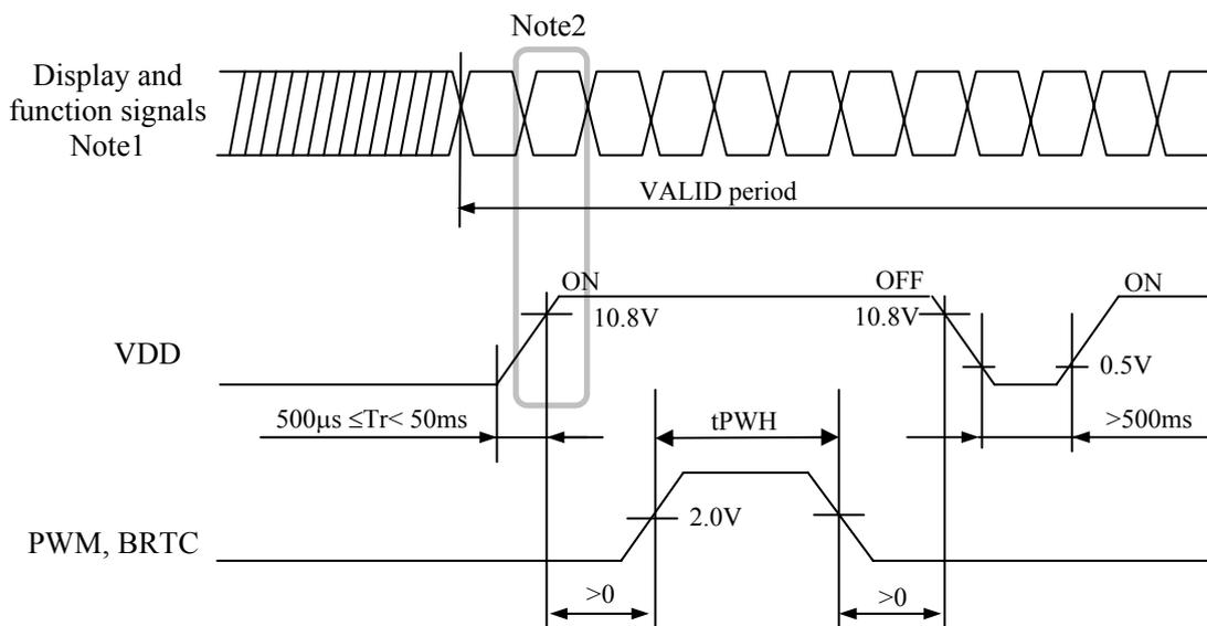
Note1: These are the display and function signals for LCD panel.
