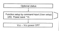
Set the time (tL) from power save to turning off the VDD - Vss power (VDD - Vss = 1.8 V) longer than the time ( $t_H$ ) when the potential of V5 ~ V1 becomes below the threshold voltage (approximately 1V) of the LCD panel. th is determined depending on the voltage
