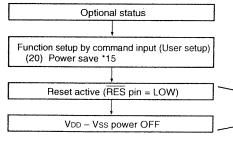
Set the time (tL) from reset active to turning off the VDD - Vss power (VDD - Vss = 1.8 V) longer than the time ( $\dot{t}_H$ ) when the potential of  $\dot{V}_5 \sim \dot{V}_1$  becomes below the threshold voltage (approximately 1 V) of the LCD panel. For th, refer to the <Reference Data> of this event. When th is too long, insert a resistor between V<sub>5</sub> and V<sub>DD</sub> to reduce it.
