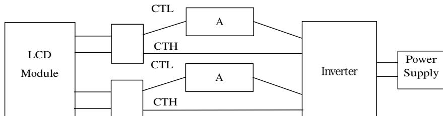
\*2) Lamp frequency of inverter may produce interference with horizontal synchronous frequency, and this may cause horizontal beat on the display. Therefore, please adjust lamp frequency, and keep inverter as far from module as possible or use electronic shielding between inverter and module to avoid the interference.
