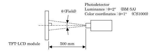
The luminance is measured according to FLAT PANEL DISPLAY MEASUREMENTS STANDARD (VESA Standard).
