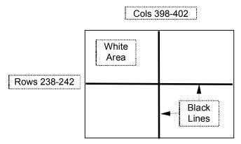
TEST PATTERN FOR IMAGE STICKING TEST
