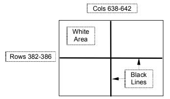
TEST PATTERN FOR IMAGE STICKING TEST
