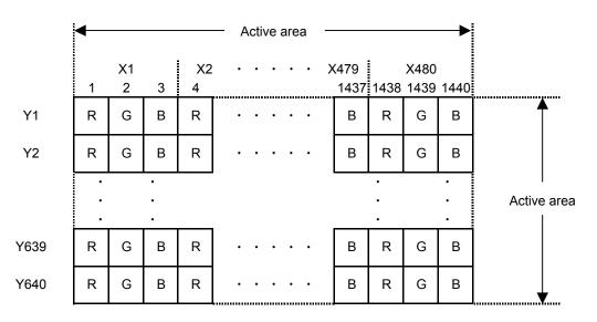
Dot arrangement (FPC cable placed left side)
