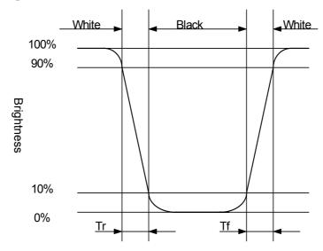
Note 12-4: Topcon BM-5A or BM-7 fast luminance meter 1° field of view is used in the testing
