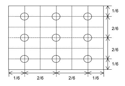
Note 12-7: Cross Talk (CTK) =  $\frac{|YA-YB|}{YA}$  × 00% YA: Brightness of Pattern A YB: Brightness of Pattern B Luminance meter : BM 5A or BM-7 fast (TOPCON) Measurement distance : 500 mm +/- 50 mm Ambient illumination : < 1 Lux Measuring direction : Perpendicular to the surface of module
